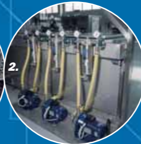
1. Extended storage weir. 2. Closed loop particle filtration with 10" cartridge filters. 3. P2S filtration system.
