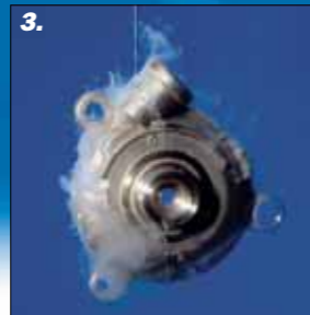
1. Air bubble agitation. 2. Dunking 80 kg. 3. Ultrasonic wash. 4. Various immersion jet or spray in air options are available.
