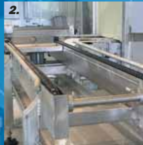
1. Transport gripping head. 2. Motorised chain conveyor for loading and unloading provides storage buffer.
