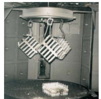
An extra feature is this revolving satellite hook which allows cleaning of delicate castings
