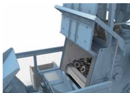
Hydraulic loading, discharge via vibratory conveyor
