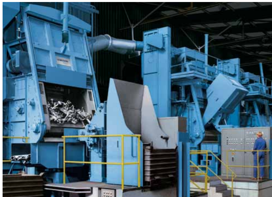
Shot blast machines in a foundry
