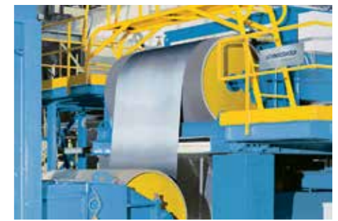
Wide strip and narrow strip after blast cleaning
