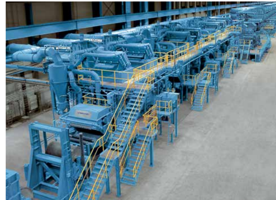
Three strip descaling machines HB-2x4/1600 operating in sequence
