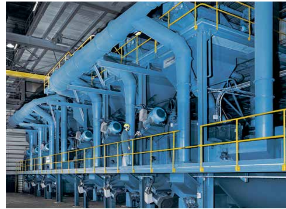
High-performance strip blast cleaning system equipped with 24 blast wheels for strip widths of up to 2100 mm
