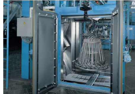
Hanger-type shotblast machine for through-feed operation
