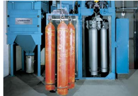
Hanger-type shotblast machine for reconditioning gas bottles
