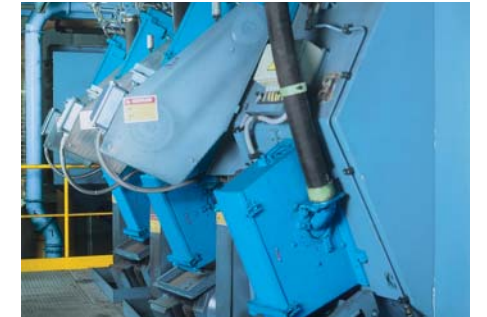
12 blast wheels, 37 kW each.
