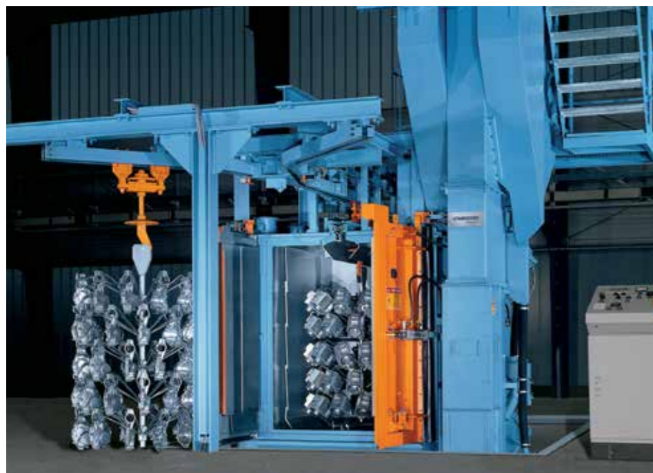
Hanger type blast machine with two blast wheels for cleaning and deburring light alloy castings
