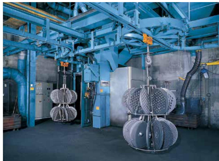
Customised monorail with switch points - hanger type machines solve blast cleaning and transport tasks at the same time.
