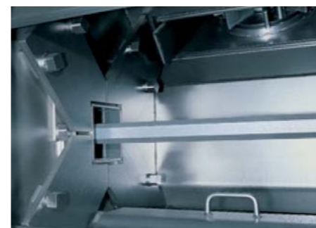
Shot blast chamber
