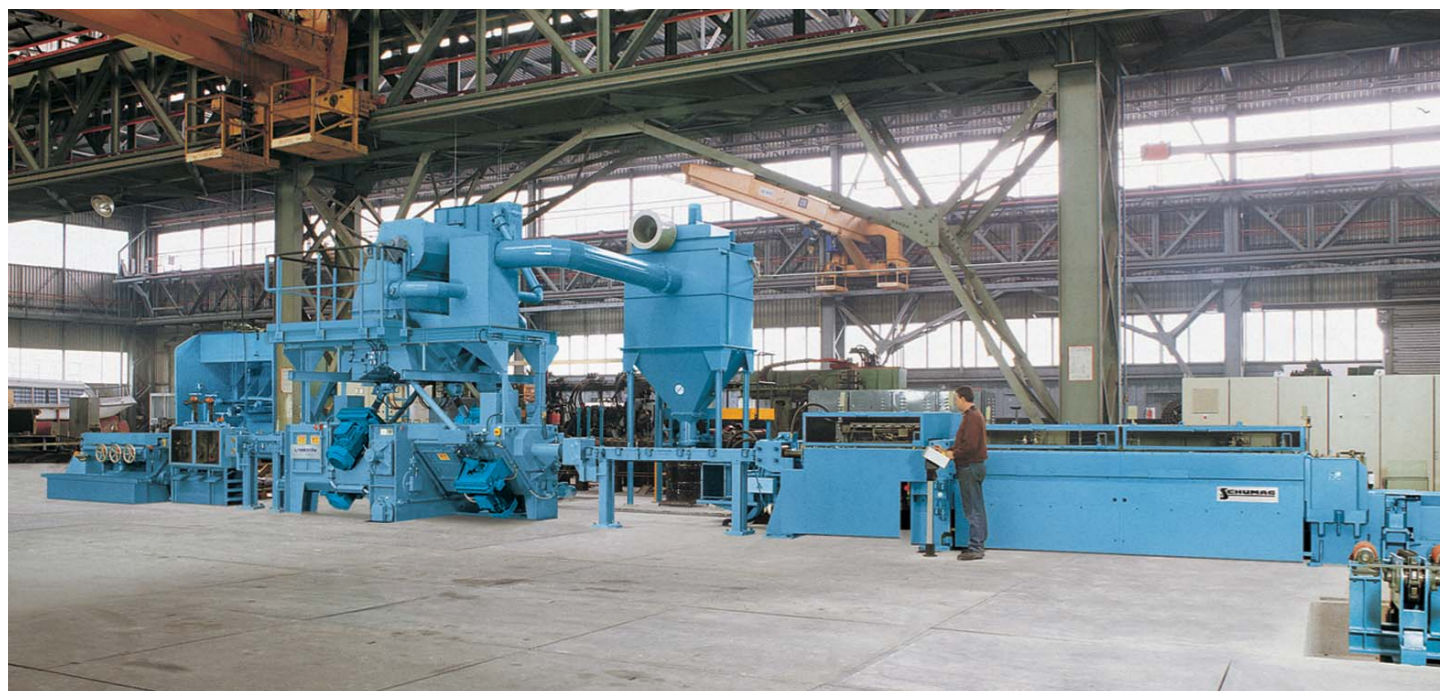
Shot blast machine with dust collector
