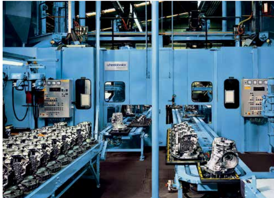
Aluminium gear boxes being blast cleaned and deburred in a DS 8 system
