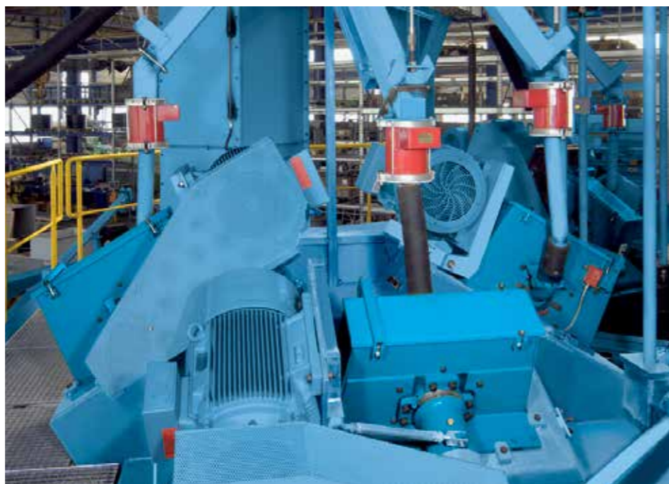
Fully automatic control of shot volume via magnetic valves
