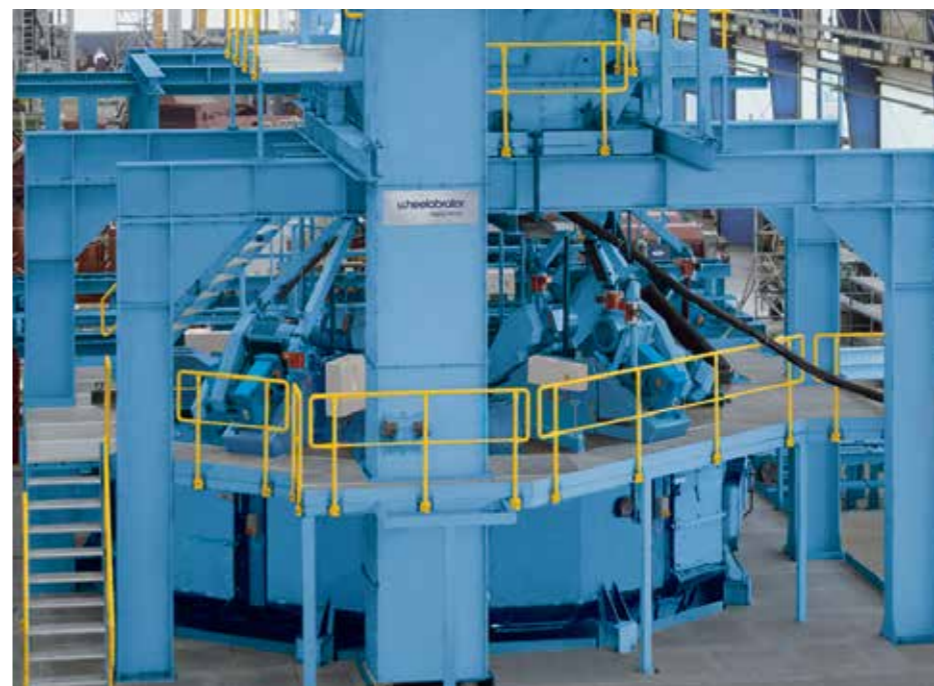
All blast wheels are conveniently accessible and coordinated for optimal shot blast results
