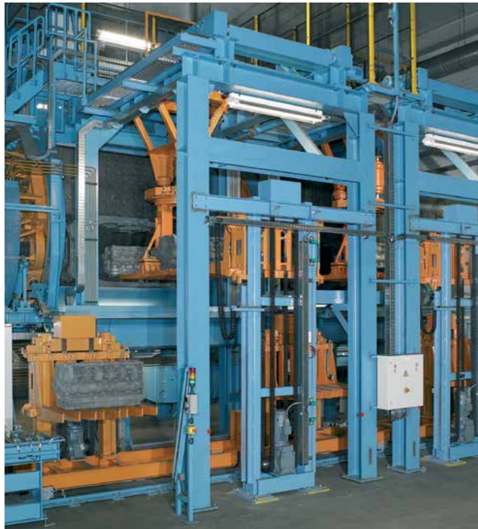
DV 4-1250 for shot blasting crankcases
