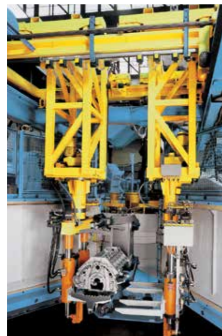
Simultaneous loading and unloading of a DS 8 via twin handling device
