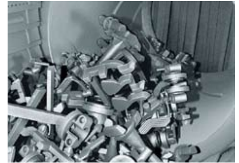
Parts in the outlet barrel after cleaning
