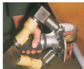
Plate edge gun. Cleans top, bottom and edge in one pass
