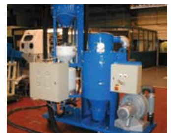
A very powerful continuous blasting P-08-2 fitted with vacuum pump recovery to reduce the air consumption
