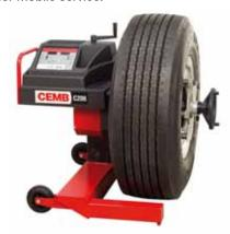
**ER80** - New balancing machine with digital panel. Completely renewed and revolutionary ergonomic design. Automatic measuring system for rims up to 30". Wheel automatic locking and indication of the correction for weight positioning by laser beam. Complete with LA Sonar for the wheel width measure. Available in both manual and pneumatic locking.
