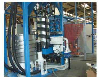
Media recovery and classification device
