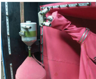
Shot flow calibration unit
