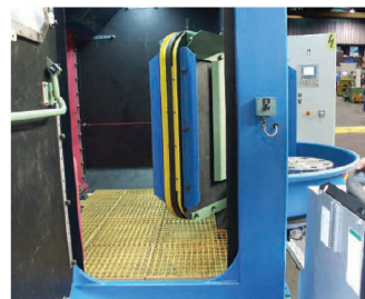
Revolving door with inflatable seal
