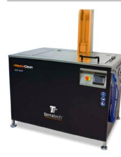
Capacity: 300 litres Useful measures: 860 x 520 x 385 mm External dimensions: 1520 x 1020 x 1030 mm Power supply: 400V Heat resistance: 7500W Ultrasonic power: 3000W (6000W p-p) Tank built in AISI 304 stainless steel of 2mm Maximum load capacity: 250kg Auxiliary tank for the separation of lubricants and oils Optional: filter for sludge and waste system Weight: 300kg
