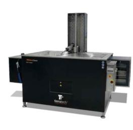
Capacity: 2000 litres Internal dimensions: 1750 x 1100 x 1080 mm Useful measures: 1650 x 910 x 790 mm Power supply: 400V Heat resistance: 2x9000W Ultrasonic power: 10200W (20400W p-p) Tank in AISI 304 stainless steel 2mm Maximum load capacity: 1000kg Auxiliary tank for the separation of lubricants and oils Optional: filter for waste and sludge system Weight: 1250kg
