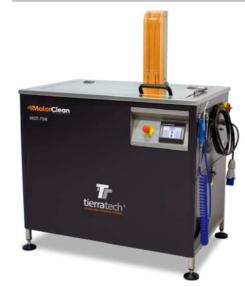
Capacity: 75 litres Useful measures: 620 x 325 x 260 mm External dimensions: 1170 x 735 x 900 mm Power supply: 240V Heat resistance: 2250W IBL, high performance titanium steel. Ultrasonic power: 800W (1600W p-p) Tank built in AISI 304 stainless steel of 2mm Maximum load capacity: 30kg Optional: filter for sludge and waste system Weight: 130kg
