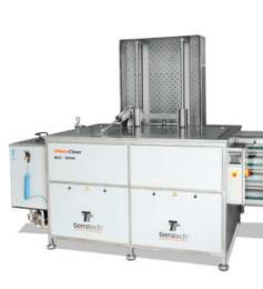
Capacity: 3000 litres Internal dimensions: 2050 x 1200 x 1205 mm Useful measures: 1930 x 990 x 880 mm Power supply: 400V Heat resistance: 2x12000W Ultrasonic power: 13600W (27200W p-p) Tank built in AISI 304 stainless steel 2,5mm Maximum load capacity: 1500kg Optional: filter for waste and sludge system Peso: 1850kg
