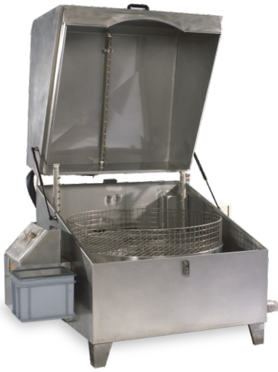
RT-series with fully opened cover provides easy access to the basket.
