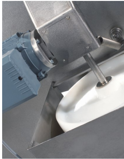
A motordrive can be fitted on the rotating basket of the toploader to ensure a positive rotation.
