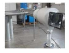
air is therefore created inside the cyclone. The solid dust particles are pushed by centrifugal action against the internal walls of the cylinder body. Gradually, and continuously, they descend to the cyclone discharge to fall inside the bin. The pressure drop in these cyclones varies between 60 and 140 mm H2O.
