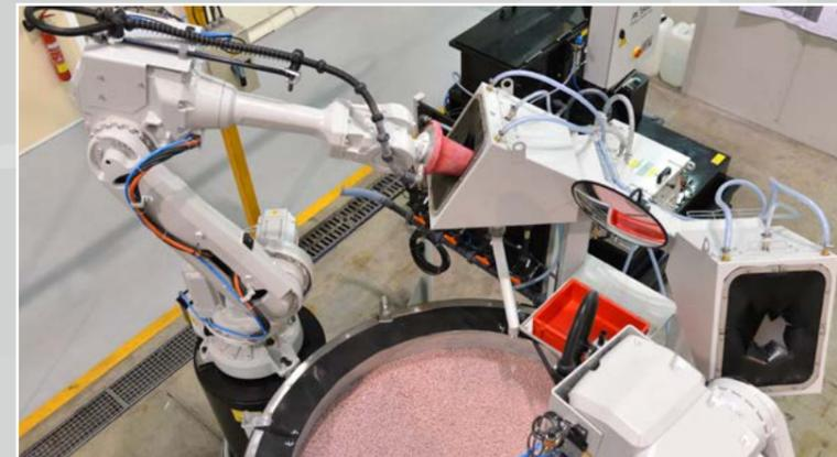
After wet, as well as dry Surf-Finishing processes the work piece surface can be contaminated with media and metal fines. The robotic handling systems move the finished work pieces to an integrated cleaning station, where they are cleaned by compressed air or process water.
