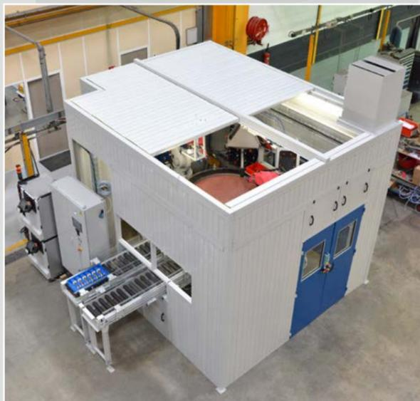
Complete system enclosures ensure compliance with safety and noise regulations.
