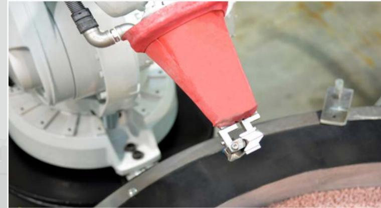
The work pieces are individually clamped to the robotic workstations. Clamping options: Work piece with internal drilled holes, direct clamping or prior mounting of the work piece to a clamping adapter.
