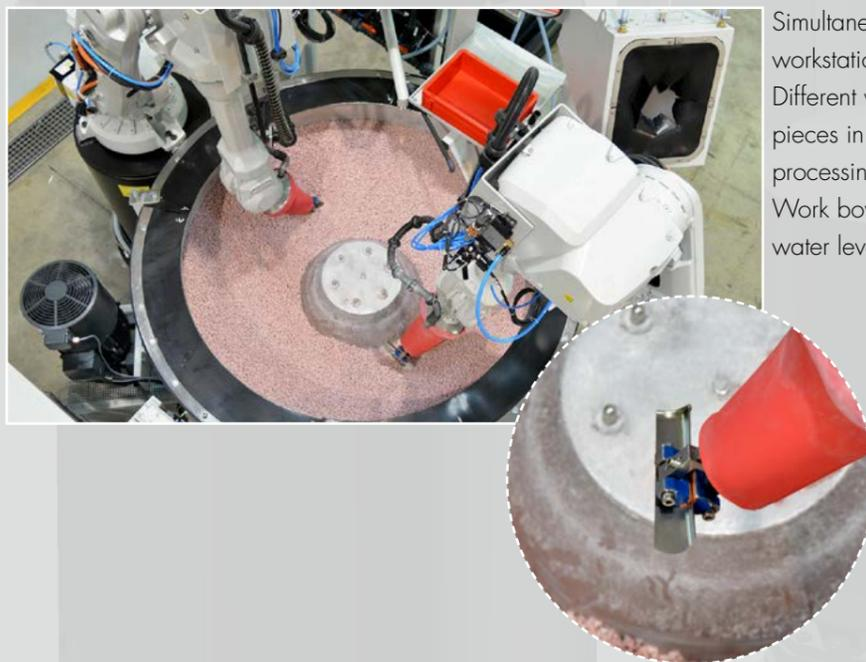
Simultaneous surface finishing with two robotic workstations. Different work piece processing options: Work pieces in stationary position, rotational movement, processing at different angles and different depths. Work bowl: Variable RPM, adjustment of the process water level
