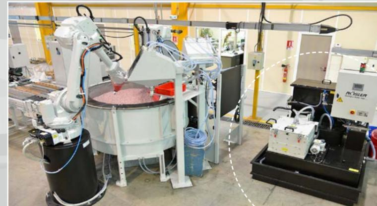
Wet processing methods guarantee clean work pieces and consistent processing results. The use of process water recycling systems saves natural resources and lowers the operating costs.
