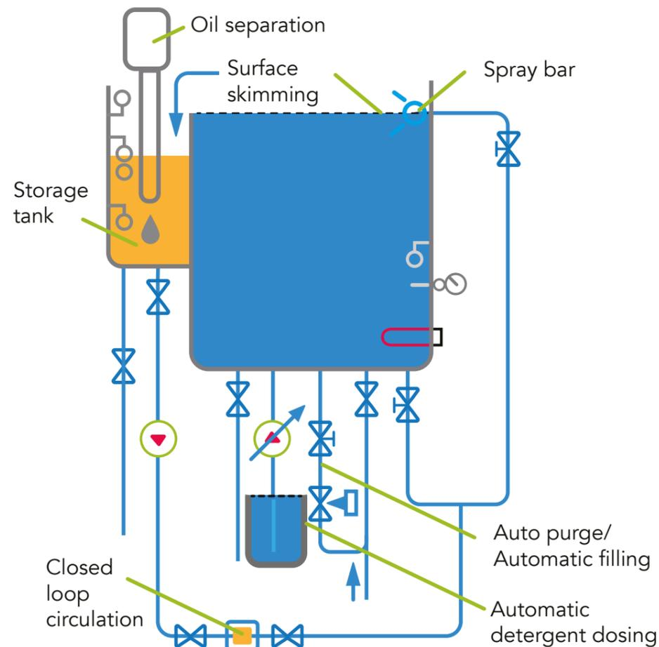
Most bath maintenance options, including the compact storage tanks, can be integrated within the encapsulation of automatic lines resulting in a more compact footprint and a cleaner look.
