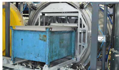
Producing and cleaning in the same goods carriers
