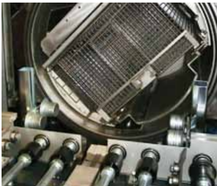
The parts movement is adjusted for optimum cleaning, based on the actual parts geometry
