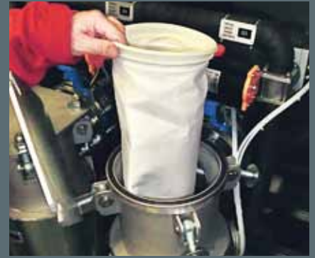
Filters with sealing collars and mesh sizes of 150 to 1 µm clean the entire solvent volume of each bath
