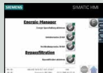
Energy-saving and filtration settings shown in the graphic display
