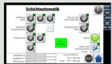
Cleaning medium, filters and distillation are maintained with simple multi-maintenance programs - the plant is maintained and ready for further operation
