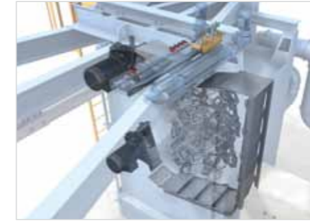
Blast cabinet with wear resistant lining
