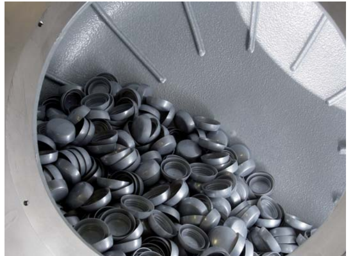
View into the drum with work pieces
