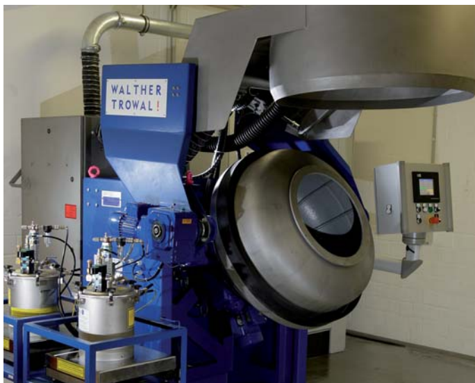
Rotamat R 90 C with opened cover
