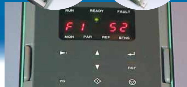
Digital panel provides user friendly control and parameter setting.
